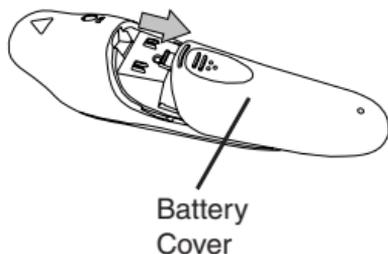
Insert the supplied battery, making sure the positive (+) and negative (-) ends of the battery match the polarity indicators inside the battery compartment.
